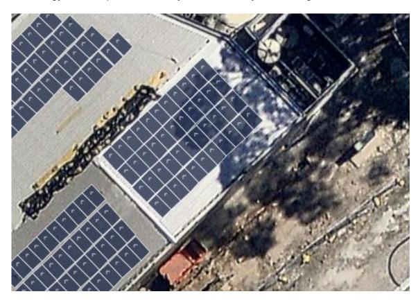
Figure 4: Shade affected North-East facing array (11kW)
