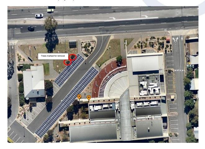
Figure 8: Proposed 55kW Carport Solar array
