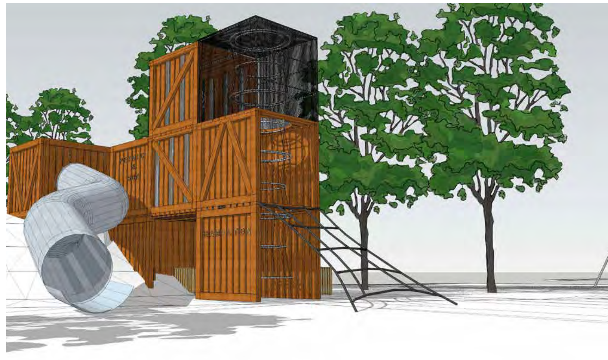
WESTERN FACADE PLAY STRUCTURE - TUBE SLIDE FORM TOP OF MOUND, SCRAMBLE NET AND INTERNAL CYLINDER NET TO CONNECT TO BIRDS NEST TOWER.
