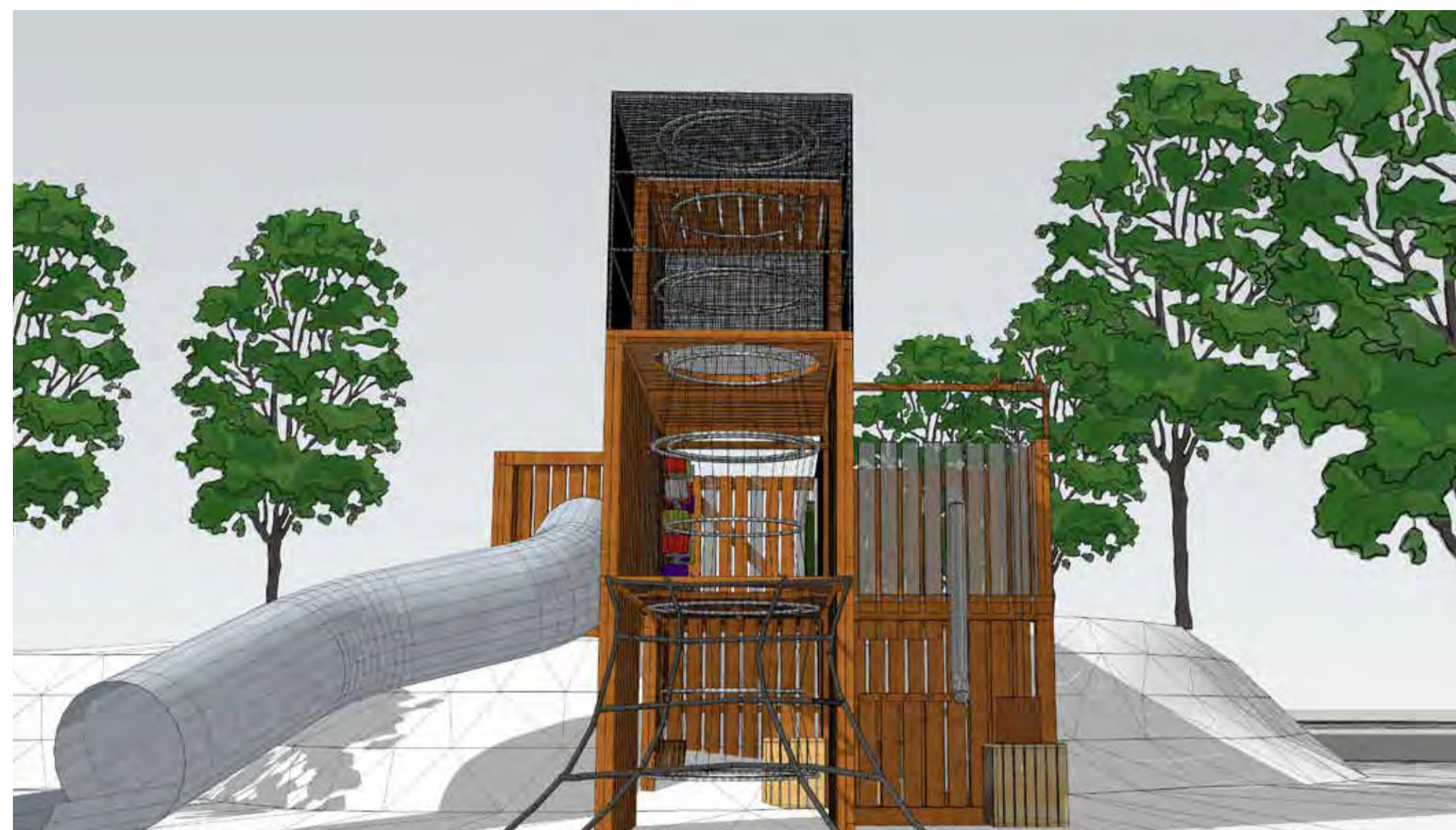
SOUTHERN FACADE PLAY STRUCTURE - BIRDS NEST TOWER ON TOP OF VINE CLIMBING STRUCTURE - EASTERN SIDE INCORPORATES CONSTRUCTION PLAY, BUCKETS AND PULLEYS TO CONNECT GROUND PLANE LOOSE PARTS
