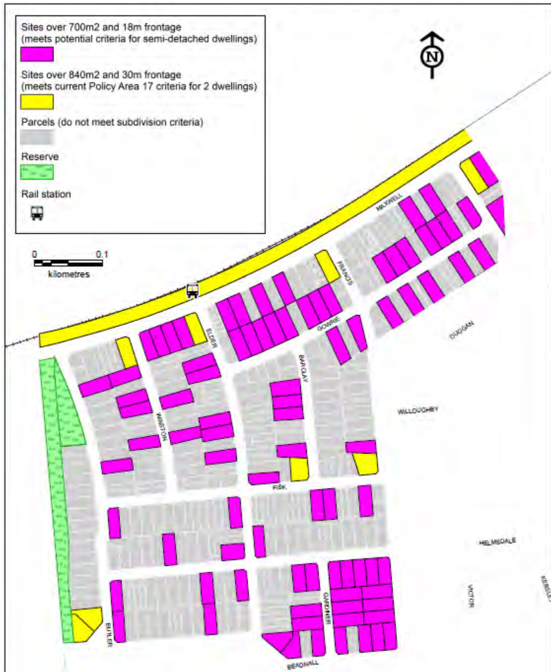
Figure 43. Development potential of amended minimum site dimensions to enable appropriately-designed semi-detached dwellings – existing Glengowrie Character Policy Area 17
