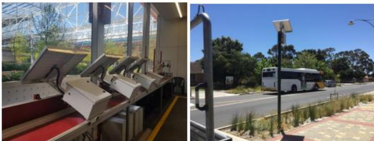
Figure 3 – Addinsight monitoring devices in construction and installed
