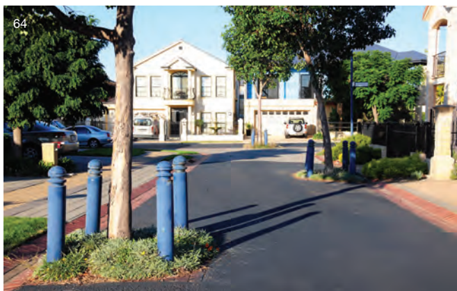
64 Position of trees shortening the line of sight and bending the vehicular path Torrens St, Mawson Lakes, Adelaide
