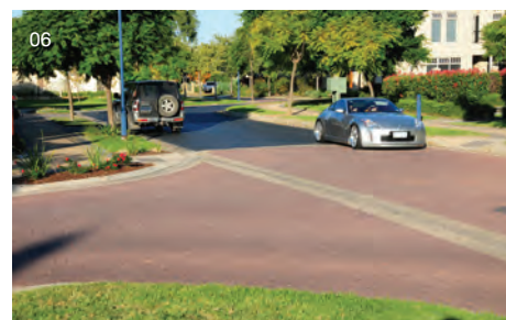
Side road entry treatments in different materials
