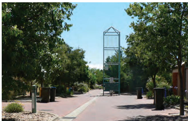
Green Lane/Park Lane/The Walkway (old MFP demonstration project), Osborne (V-E) Residential precinct for some 60 dwellings with shared zone roadways for 2-way traffic access, no separation of road users in roadway, marked angled parking and many plantings
