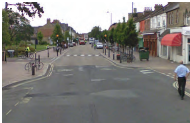
Cowley Rd, Oxford (UK) (III-C) District shopping centre street located on a secondary route into the centre, which accommodates two lanes of traffic, limited parking and level surface crossing points for pedestrians
