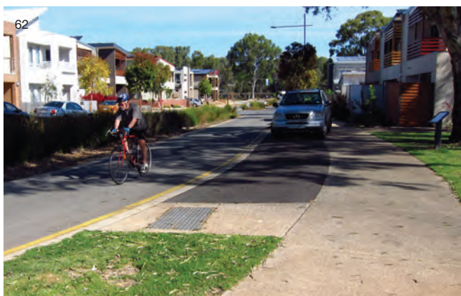
62 Horizontal deflection (bending road) and visual carriageway narrowing through landscaping Lochiel Parkway, Campbelltown, Adelaide
