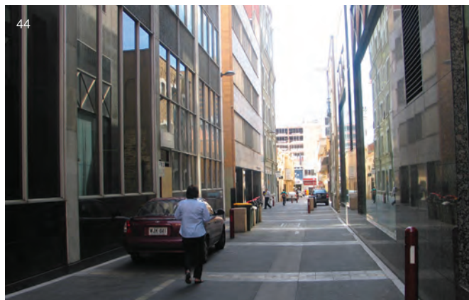
Peel Street, Adelaide (V-E) Single lane for vehicles delineated by large bollards and parking areas
